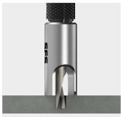
The geometry of the drill hole shall be checked minimum on 1% of all drillings. **Nominal measure:**  $\emptyset$  **5.9 – 6.0 mm** (Can be measured with a vernier caliper)
