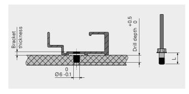
For CNC milling, a milling cutter  $\emptyset$  6.0 mm with tolerance h6 is recommended
