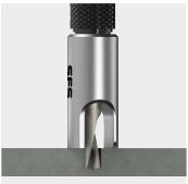
The geometry of the drill hole shall be checked minimum on 1% of all drillings. Nominal measure: Ø 5.9 – 6.0 mm (Can be measured with a vernier caliper)
